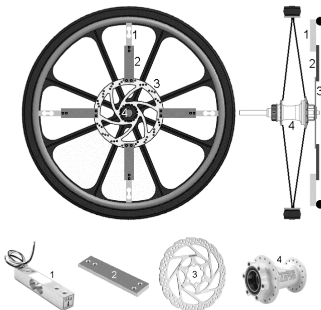
Figure.1: Top drawings: assembled handrim prototype inside and front views. Bottom drawings: mechanical used spare parts.
