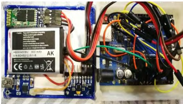
Fig. 4. The Wobble Box disassembled. Left up is the HC-06 Bluetooth module. On the bottom left is the TP4056 Li-ion battery charger. In the middle is the Inertial Motion Unit MPU6050 and on the right the Arduino board. The batteries on the left gives an output of 7,4V.
