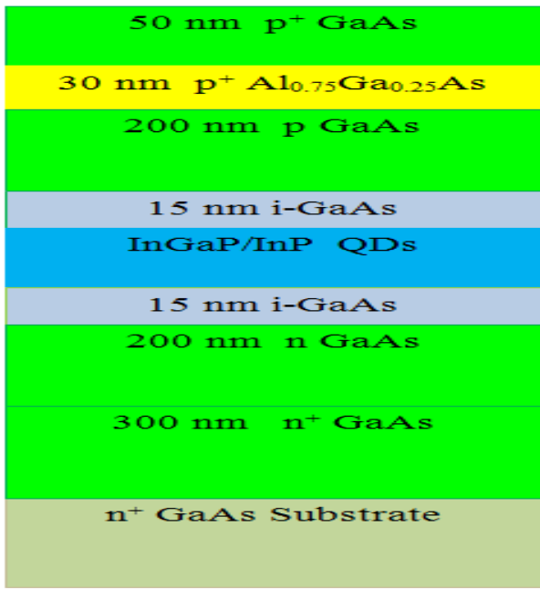
Figure.1: Structure of InP/InGaP quantum dots solar cell.
